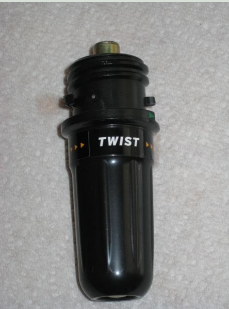
Illustration 2: The two tabs just below the threads should be cut off
