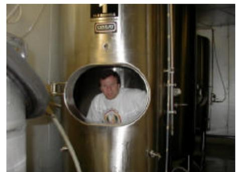
Meanwhile, Stacy helped Scott assemble the plate filter. We cleaned the now empty serving tank, which involved rinsing any residue of the Cherry Porter out of the tank and then climbing inside with a scrungie pad to wipe down the walls. After another rinse the tank was sanitized in the same manner as the fermenter.
